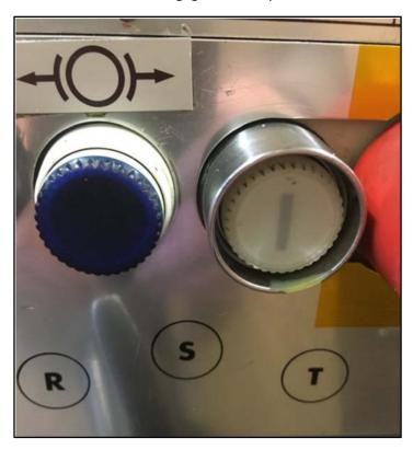
The switch is located next to the main motor switch to the left of the coolant pump switch. When it is actuated a light shows in the switch. Pressing it again locks the brake & the light goes out.
