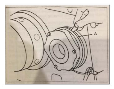
The illustration is somewhat disingenuous because it shows the brake unit mounted to the outside surface of the headstock whereas it is embedded into a counterbored recess & access with the feeler gauges is severely limited.
