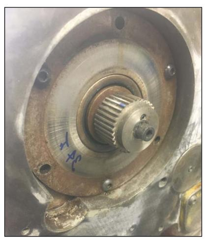
The Friction Plate slides on the splines.
