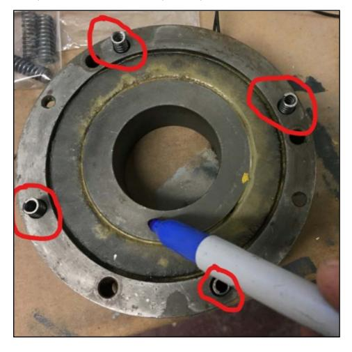
**To reassemble**-after ensuring that the friction surface on part 71265-1-Housing is grease free, slide the friction plate onto the splined hub. Then the pressure plate can be fitted over it. Ensure that the cut-outs indicated are positioned as shown where the 3 fixing screw holes are located. No friction plate is fitted in the view shown. It should be sandwiched between the pressure plate & the housing.
