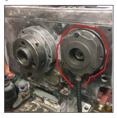
**Remove the 3 cap screws** & this is what you see. The following description is of an Ortlinghaus brake. I understand that the Matrix part is broadly similar.
