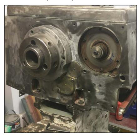
**Close-Up Detail** showing the splined centre which is keyed to the output shaft. The Ortlinghaus splines measure 35mm outside diameter whereas those on the Matrix are 40mm diameter.
