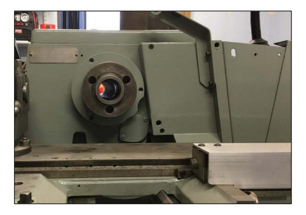
To remove it you first must unscrew & lift away the splashback. The triangular sheet metal part can then be unbolted & placed to one side before unscrewing the brake cover.
