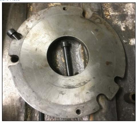
Which is actuated by the springs shown circled below on the view of the 'inside' of the brake housing. The pen is pointing to the pole of the electromagnet which attracts the pressure plate away from the friction plate to allow it to rotate independently.
