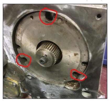
The brake housing complete with springs & the tubular spacers fitted over the pre-inserted Allen fixing screws can then be offered into place. Locate the screws into the tapped holes & progressively tighten against the headstock which will compress the springs. Alternatively, 2 M6 screws can be used in the opposing holes one of which is marked below to screw into the pressure plate to compress the springs before offering the brake up to the headstock.
